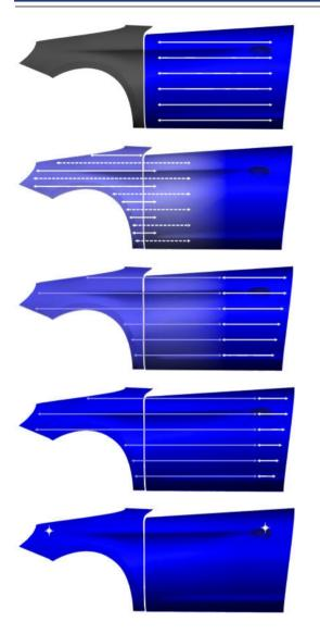
Adjacent panel: sand panel with suitable abrasive e.g. Trizact – P1000. New part / repair: sand filler (minimum P500).
